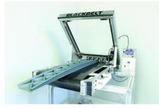
The Blackbelt 3D printer is a new type of 3D printer using fused filament fabrication (FFF) in combination with innovative belt technology. Printing on a belt (patent pending) provides new possibilities like long prints, printing horizontal overhangs without support and producing series production of the same or individual parts.
