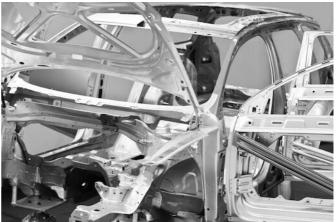
To provide increased passenger safety, and simultaneously comply with emissions legislation, future vehicles must be stronger and yet lighter. Each new vehicle model therefore contains a higher proportion of modern, high strength steel than its predecessors. To ensure high productivity when forming these demanding steels, especially resilient coating solutions are required – such as BALINIT<sup>®</sup> FORMERA.
